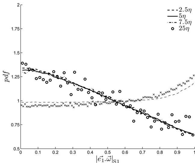
FIG. 4. *pdf* for the magnitude of the alignment cosine between  $\mathbf{e}_1$  and  $\boldsymbol{\omega}$  in sector S1 of the  $Q$ - $R$  plot of Fig 2. The dashed line and the crosses are the global *pdfs*, across all four sectors, for the data filtered at 2.5 and 7.5 $\eta$ , respectively.
