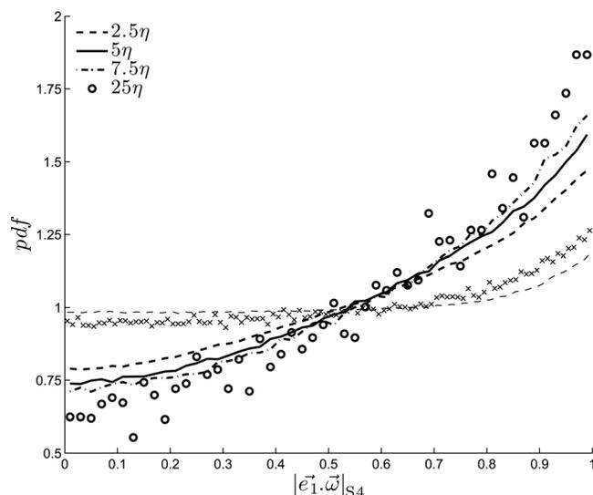
FIG. 3. Probability density function ( $pdf$ ) for the magnitude of the alignment cosine between the extensive strain-rate eigenvector ( $\mathbf{e}_1$ ) and the vorticity vector ( $\boldsymbol{\omega}$ ) in sector S4 of the  $Q$ - $R$  plot of Fig 2. The dashed line and the crosses are the global  $pdfs$ , across all four sectors, for the data filtered at  $2.5$  and  $7.5\eta$ , respectively.
