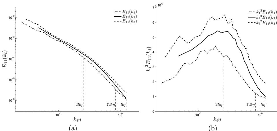
FIG. 1. (a) Mean power spectral density as a function of wavenumber ( $E_{11}(k_i)$ ). (b) Mean dissipation spectrum as a function of wavenumber ( $k_i^2 E_{11}(k_i)$ ). The three filter widths greater than the Nyquist frequency used in this study are illustrated on the figures.
