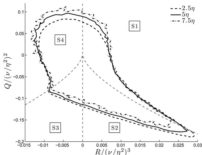
FIG. 2. Joint probability density function ( $pdf$ ) between the second invariant ( $Q$ ) and the third invariant ( $R$ ) of the characteristic equation for the velocity gradient tensor. The dashed lines mark  $R = 0$  and  $D = 0$ , where  $D$  is the discriminant of the characteristic equation.
