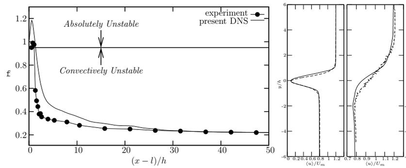
**Fig. 5.** Left: Longitudinal evolution of the wake deficit parameter  $f(x) = (U_m - \min_y[\langle u \rangle(x, y)]) / U_m$ . Centre: Comparison of the mean velocity profile at  $x-l = 1.6h$  (solid line) with the generic profile used by [13] (dotted line). Right: Comparison of the mean velocity profile at  $x-l = 42h$  (solid line) with its experimental counterpart [3].
