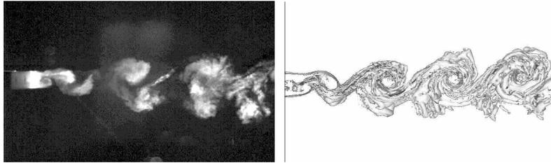
**Fig. 4.** Experimental (left, [3]) and vorticity (right, present DNS) visualizations of the TML.
