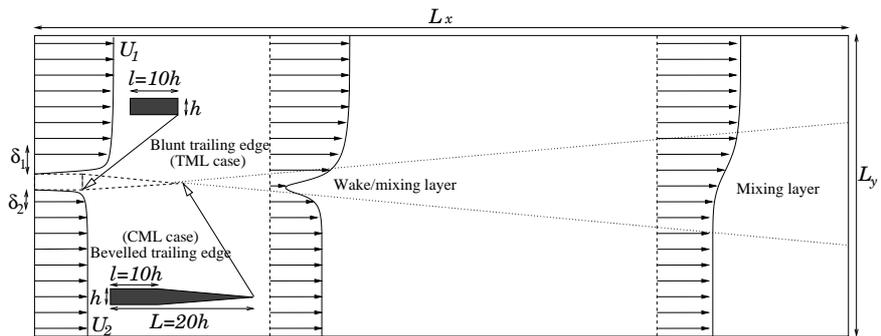
Fig. 1. Flow configuration and computational domain.
