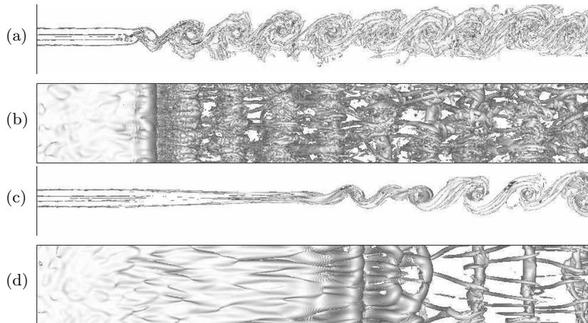
**Fig. 3.** Vorticity isosurfaces for DNS 3D results. TML (top) and CML (bottom) cases in side or upper views.
