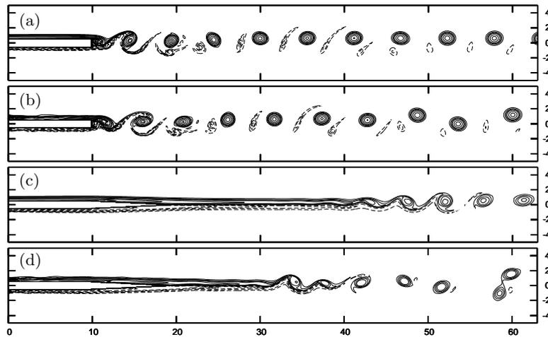
**Fig. 2.** Vorticity contours for DNS 2D results (dashed lines indicate positive contours). TML (ab) and CML (cd) cases with (bd) or without (ac) inflow perturbations.
